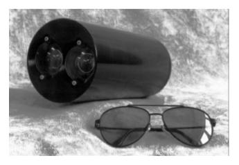
Figure 1: The compact underwater stereoscopic video camera.
