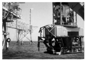
Figure 3: The Triton ROV fitted with the stereoscopic video system at the North Rankin Platform
