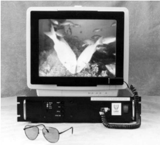
Figure 2: The stereoscopic display
