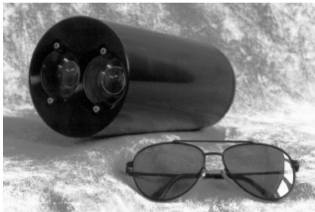
Figure 1: The compact underwater stereoscopic video camera.
